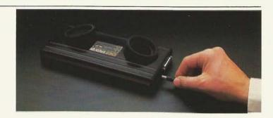
Plug the 25-pin connector of the modem cable into the 25-pin connector port on the right side of the modem.
