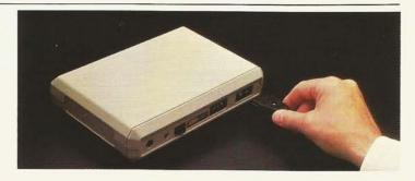
Plug the other end of the I/O cable into the connector port on the computer or other peripheral (except the ATARI 410<sup>™</sup> Program Recorder or ATARI 825<sup>™</sup> Printer).
