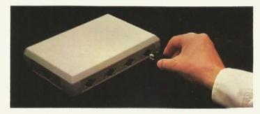
Plug the interface module's I/O cable into one of the front connector ports on the interface module.
