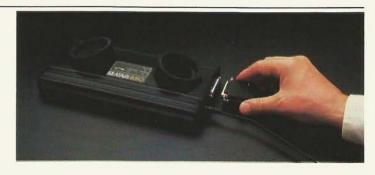
Plug the other end of the modem connector cable into SERIAL PORT 1 of the interface module.
