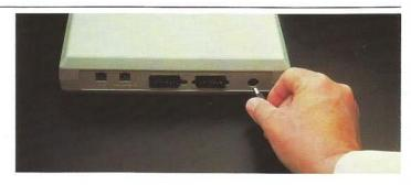
Plug one end of the direct connect modem I/O cable into one of the rear connector ports on the modem.
