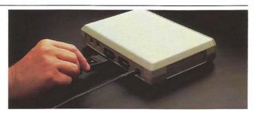
Plug the other end of the I/O cable into the connector port on the computer or other peripheral (except the ATARI 410<sup>™</sup> Program Recorder or ATARI 825<sup>™</sup> Printer).
