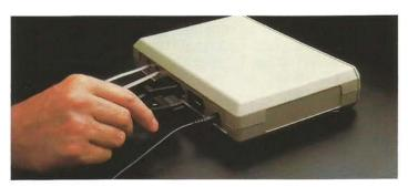
Pull the door release forward on the computer to open the cartridge door.
