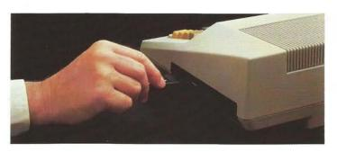
4 Unplug the telephone from its wall jack. Plug the telephone cord into the jack labeled TELEPHONE on the back of the ATARI 835 Direct Connect Modem.
