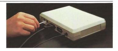
Plug one end of the telephone cord supplied in the kit into the jack labeled LINE on the direct connect modem. Plug the other end into the telephone wall jack.
