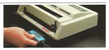
Plug a connector cable into a connector port on the front of the interface module. Plug the other end of the cable into the unused connector port on the back of the direct connect modem. Refer to the ATARI 850 Interface Module Operator's Manual for more detailed setup instructions. Turn on your TV.
