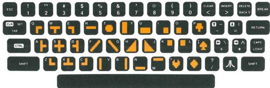
Figure 4 Screen Control Graphics Keyboard Diagram
