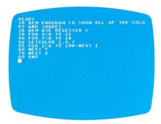
Experiment with SETCOLOR on Register 1 to determine the shade of the letters on the screen. If the letters disappear while in the direct command mode, press the SYSTEM RESET key.
