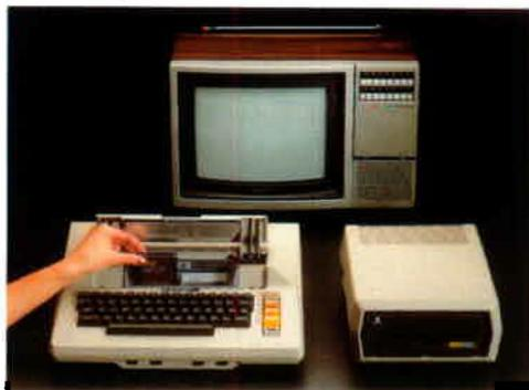
**2** Turn the disk drive on. When you first turn on the drive, it makes a whirring sound. After a moment the whirring stops and the BUSY light goes out, but the PWR ON light remains on.
