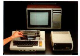
Remove the ATARI Master Diskette II from its protective sleeve and insert it into the disk drive with the label facing up. Then close the door.
